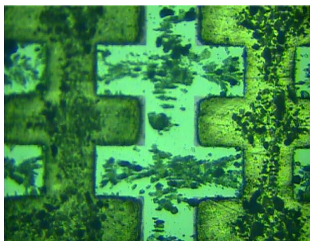
Fig. 10. Magnified view of particle distribution 5 s after voltage is applied to the electrodes.
